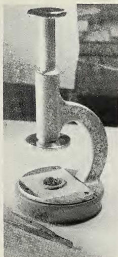
Fig. 1. Press used to obtain plasticine block impressions.
